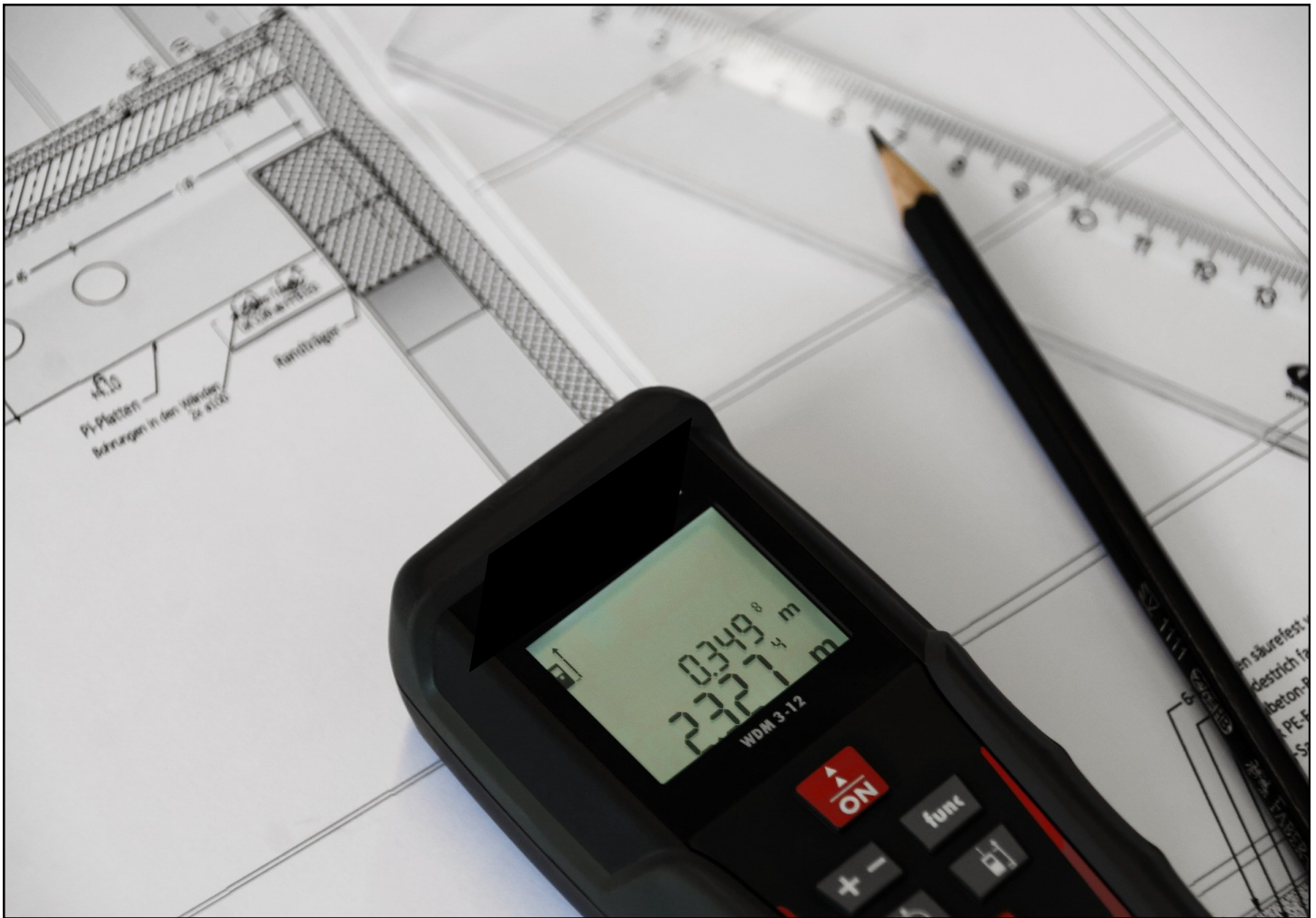
Figure 8. Using a laser measure takes the guesswork of measuring a room. They are accurate, easy to use, and cost-effective.
